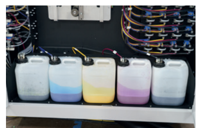
Bulk feed for greater ink cost efficiency.
